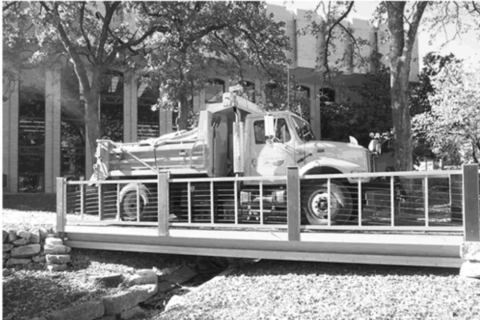
Figure 1 Load test of the UMR smart composite bridge
